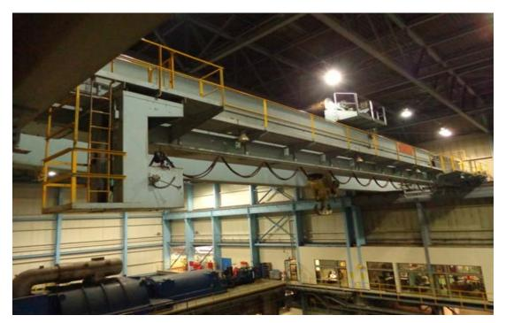
Figure 1: Overhead Crane<sup>1</sup> in Holyrood Powerhouse Turbine Hall
